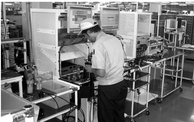
Photograph 12: Small-sized R series Workflow from sensor characteristic inspection to label printing/issue
