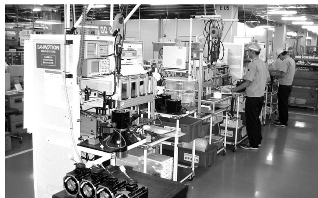
Photograph 10: Medium-sized R series sensor adjusting and inspecting line
