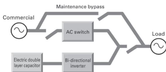
Fig.3: Basic circuit configuration of the “SANUPS C23A”
