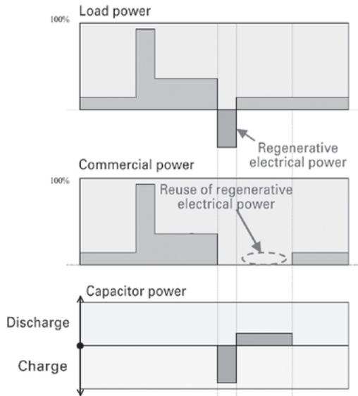
Fig. 8: Power pattern when regenerative electric power is generated
