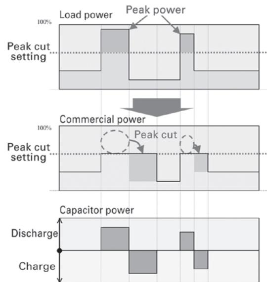
Fig. 7: Power pattern during peak cut operation
