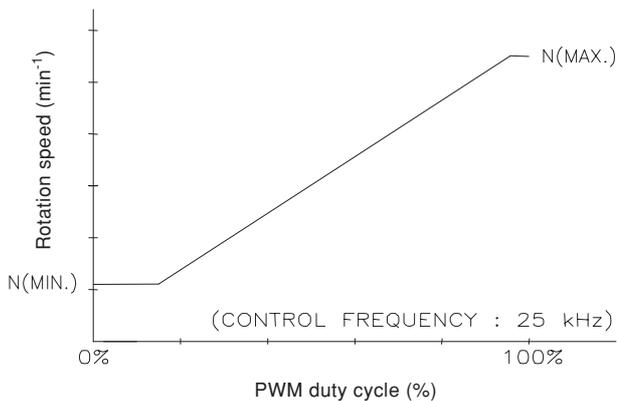
Fig. 4: Example of PWM specifications
