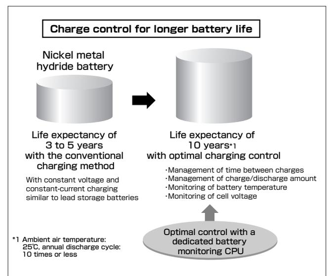
Fig. 3 Elements of optimal charging control.
