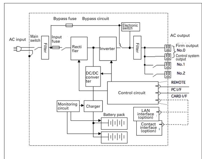
Fig. 4 "SANUPS A11G-Ni" circuit system diagram
