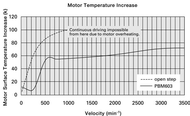
Fig. 6: Motor Temperature Increase (during No-Load Continuous Operation)
