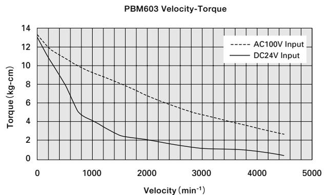
Fig. 7: Comparison of velocity-torurue characteristic
