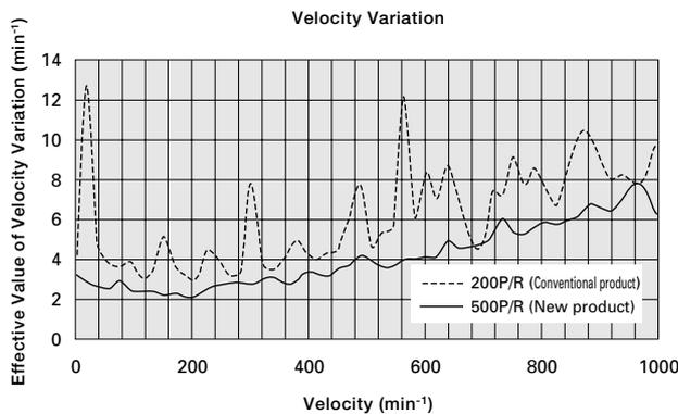
Fig. 4: Comparison of Velocity Variation (Equivalent to PBM603)
