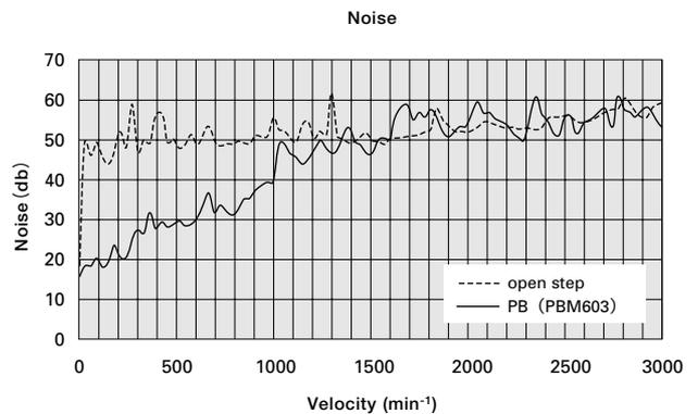
Fig. 5: Comparison of Motor Noise (Equivalent to PBM603)
