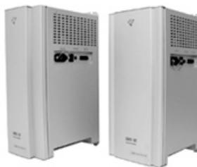
The "SMS-30" uses AMD's K6™-2E 233MHz as a CPU and an NLX bus (ISA/PCI) as an internal bus. This will hopefully expand our business of HMI and other solutions.
