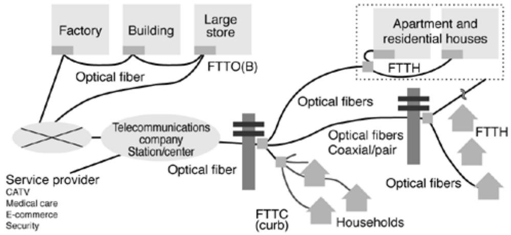
Fig. 2 Positioning of FTTH
