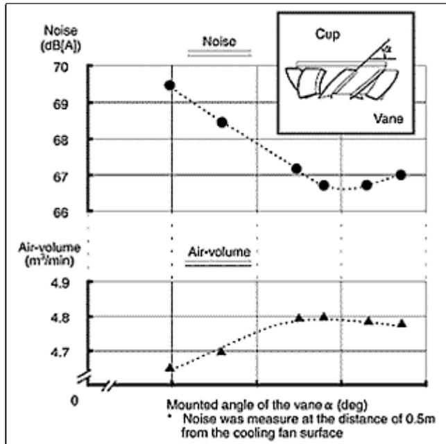
fig. 4 Mounting angle of the vane and noise/air volume
