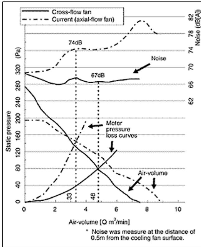
fig. 5 Air volume and noise characteristics of the current(axial-flow) fan and the cross-flow fan
