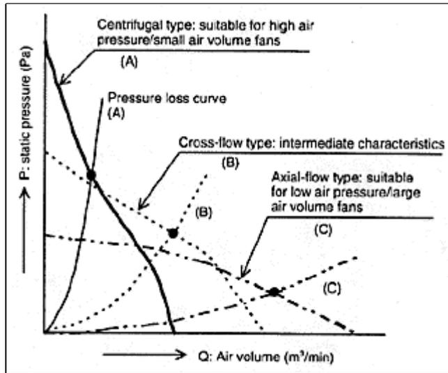
fig. 1 Type and Static pressure/Air volume characteristics of cooling fan
