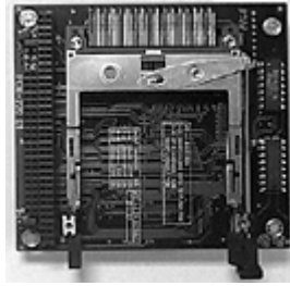
Fig. 3.7 External appearance of PCMCIA module
