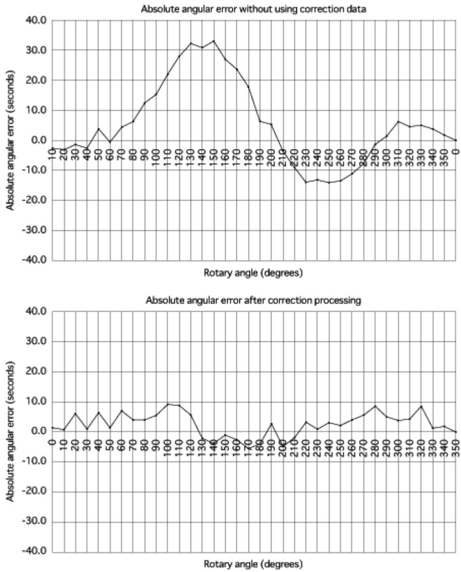
**Fig. 4 Example of evaluation data of an actual machine**
