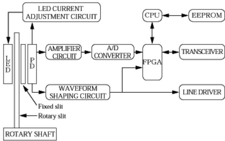
**Fig. 7 Outline block diagram of high-accuracy, high-resolution ABS-EC**
