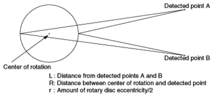
**Fig. 1 Relation between amount of eccentricity and amount of jitter**
