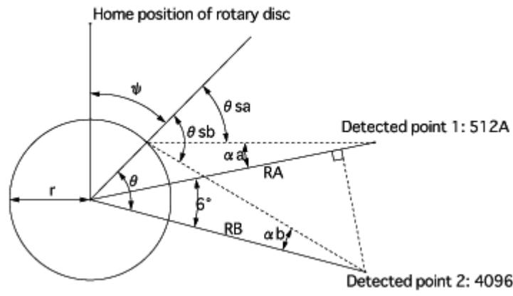
**Fig. 3 Relation between eccentricity and absolute error**
