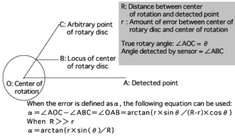
**Fig. 2 Relation between jitter and absolute error**
