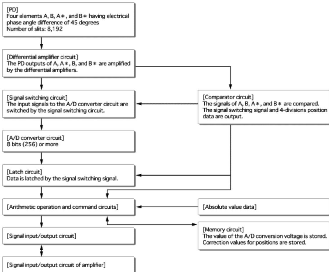
**Fig. 5 Circuit Block Flow**
