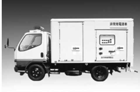
Fig.1 Outside view of "Mobile Power Supply System"
