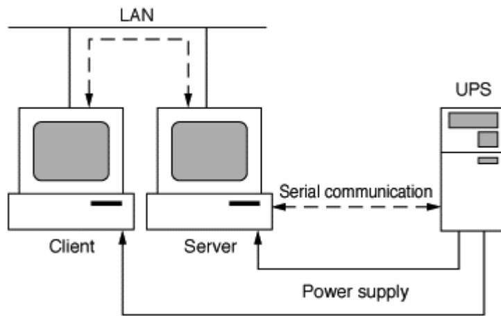
Fig.7 Configuration example using SNMP card
