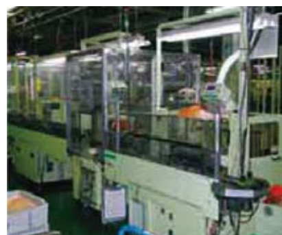
Lead-free high-temperature soldering equipment at the Fujiyama Works
