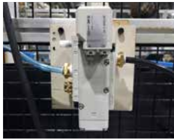
Reduction of blow time through pulse blowing
