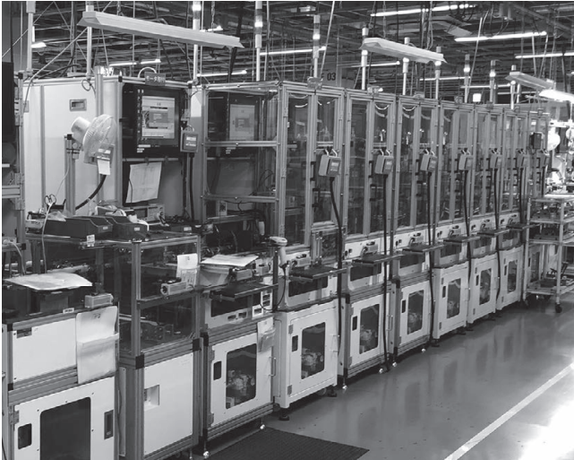
Fig. 10 Automated production line for DC servo motors
