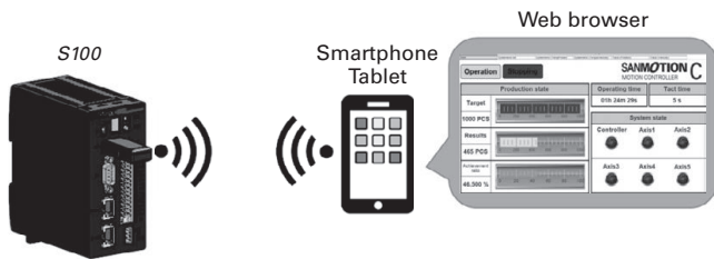
Fig. 6 Visualization of production equipment conditions
