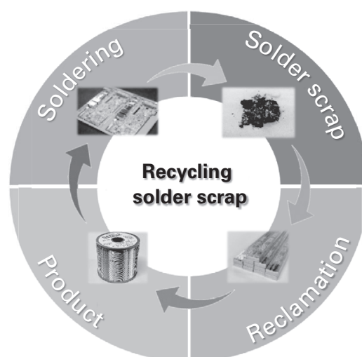
Fig. 8 Flow of solder scrap recycling
