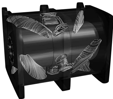
Fig. 6 Simulation example (Airflow of the new product)
